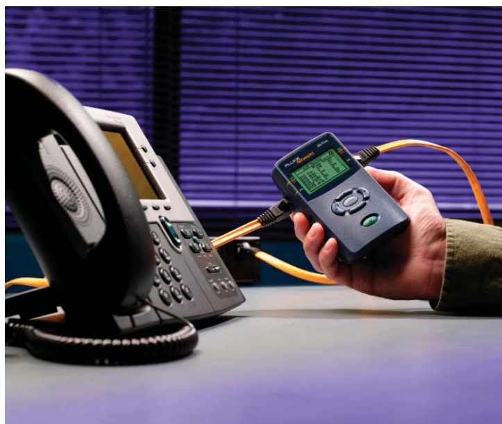
An inline network test tool is easy-to-use, affordable, and goes in-room with the BMET to the point of the problem.
